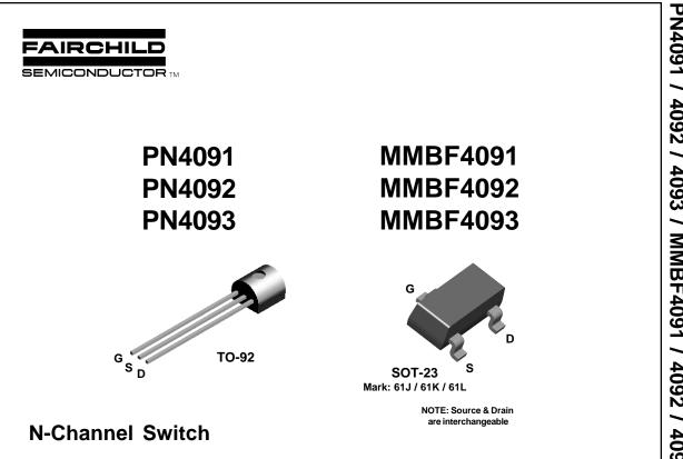
This device is designed for low level analog switching, sample and hold circuits and chopper stabalized amplifiers. Sourced from Process 51. See J111 for characteristics.
